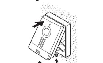
Insert the top section of the video door station into the mounting frame and push in the bottom section. Tighten the locking screw on the bottom to secure the video door station.
