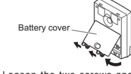
Loosen the two screws and remove the battery cover.
