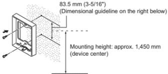
Secure the stand using the two included screws or wooden screws.
