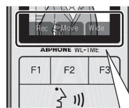
The functions displayed on the screen can be manipulated by the function button just below.
