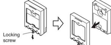
Loosen the locking screw on the bottom and remove the frame.
